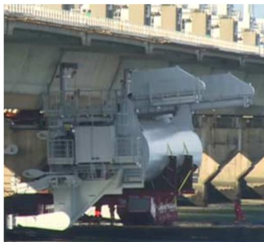
The turbines consist of a permanent magnet direct drive generator and patented bi-directional reversible rotor blades design, developed, manufactured and installed in close cooperation with major industry partners.
