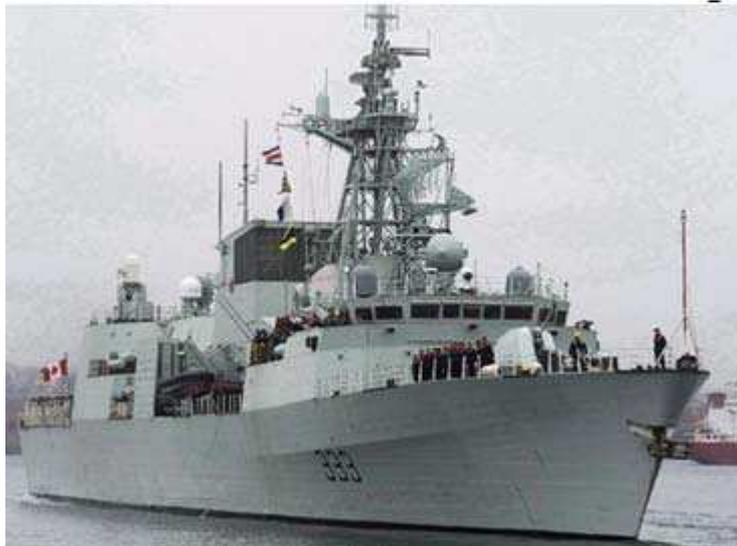
“The frequency and intensity of the tonals generated would allow acoustic sensors to both detect and identify the ship at ranges well in excess of the norm for the **Halifax Class**, and could also render the ship more vulnerable to acoustic-homing weapons,
